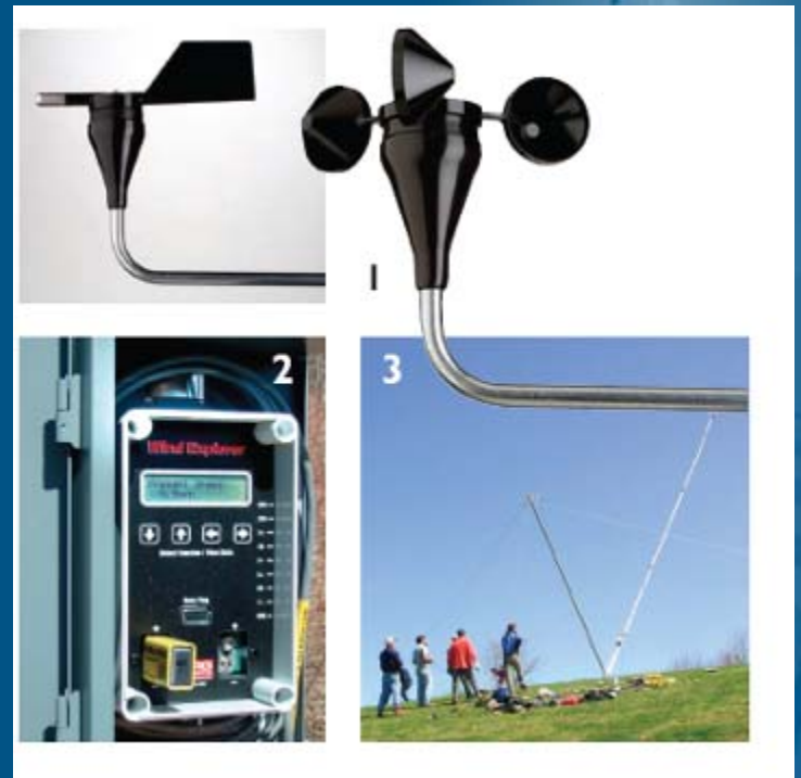
1)Anemometer and Wind Direction Vane 2) Datalogger 3) MetTower
