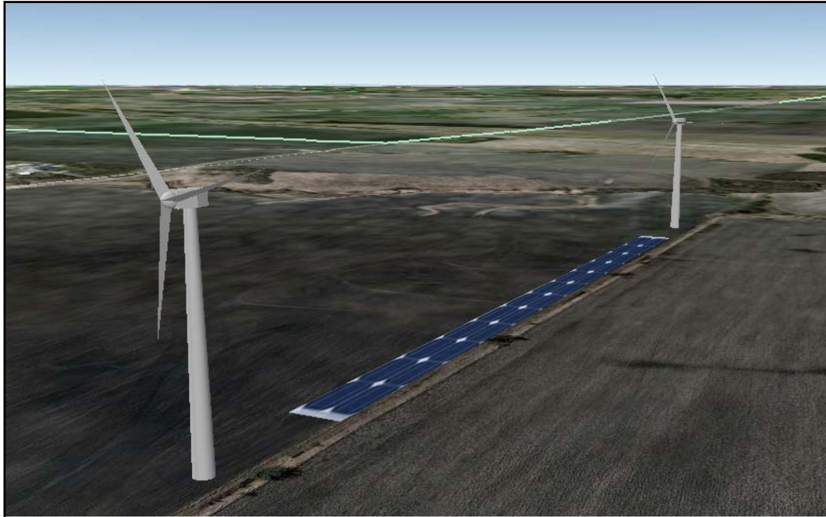
Two GE 1.7 MW WTG's & 1.5 MW of Solar Array
