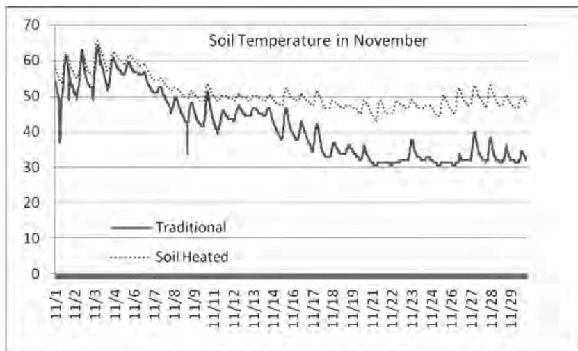
**Figure 8.** Soil temperature (2 inches) in the traditional and soil-heated high tunnels during the month of November. We used an electric air heater in both tunnels from November 1-15. We shut the electric heater off in the traditional tunnel on November 16 and kept the air heater on all month in the soil-heated tunnel.
