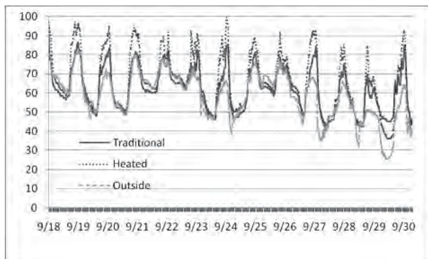
**Figure 6.** *Temperature in the soil-heated and traditional high tunnels before the heating system was hooked up. Nighttime temperatures were similar in the traditional high tunnel and the new high tunnel, except during the heavy frost on September 30, when the temperature in the new high tunnel was lower than the traditional high tunnel.*
