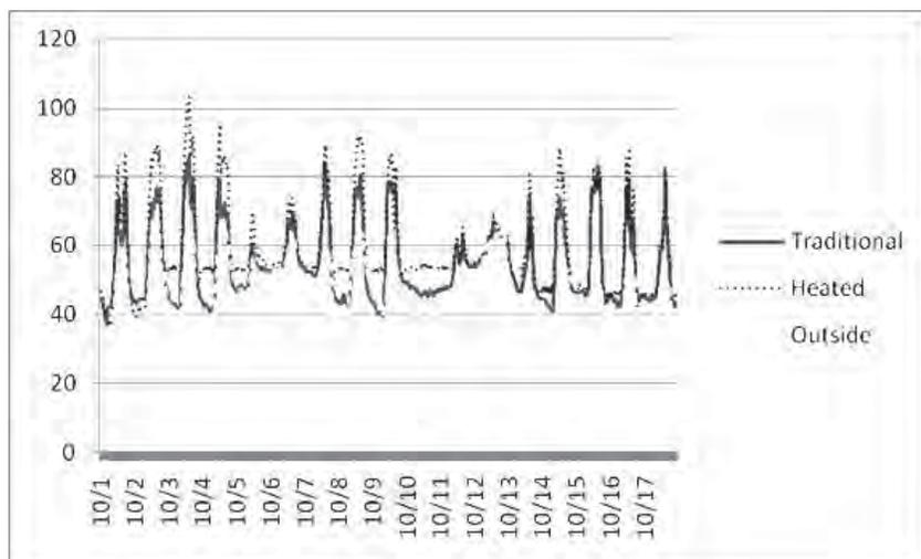
**Figure 7.** Air temperature in the soil-heated and traditional high tunnels in October. Neither high tunnel had supplemental heat. The temperature in the soil-heated high tunnel dropped to 53°F each night from October 3 through October 12, regardless of the outside temperature.
