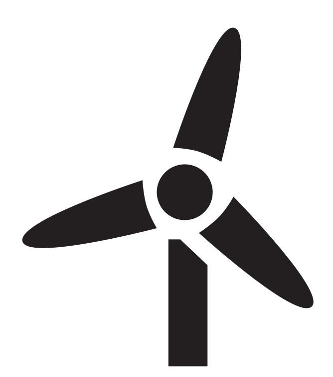
Just like a windmill, wind turbines like this one use blades to collect the wind's kinetic energy. The wind flows over the blades, which causes them to turn. The blades are connected to a drive shaft that turns an electric generator to produce renewable electricity.
